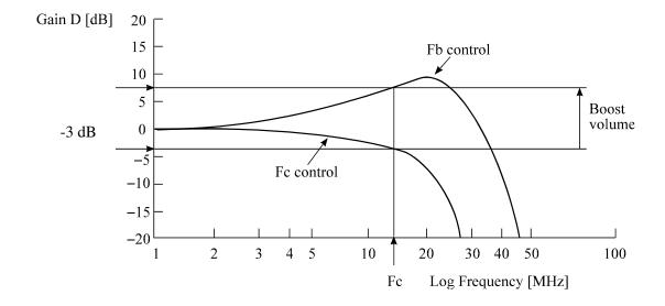
Figure 4.5 Frequency characteristic of programmable filter
